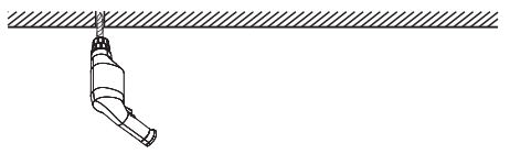
1. Drill a \varnothing 6\text{mm} hole
